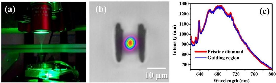
**Figure 1. Optical waveguide fabrication in diamond.** Femtosecond laser focused below the surface of a diamond sample (a) is used to write two modification tracks separated by 13  $\mu\text{m}$ , being the optical mode is guided between these two lines (b). The  $\mu$ PL spectrum inside the waveguide is the same as the pristine diamond (c), demonstrating preserved nitrogen vacancy properties, crucial for applications in quantum computing and magnetometry.
